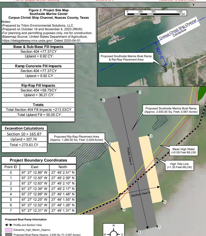
SWG-2008-00486 Proposed Construction of the Southside Marine Center Boat Ramp
